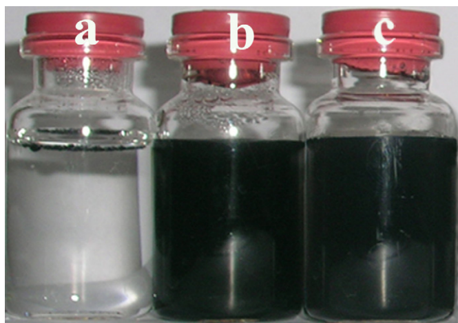
Fig. 2. Dispersion of (a) raw-MWCNT, (b) o-MWCNT and (c) e-MWCNT in water at a concentration of 1 \text{ mg mL}^{-1} .
